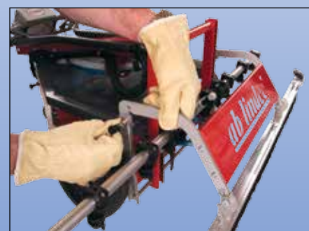
To change or remove the tool, pull out the bolt's on both sides and lift straight up simultaneously.
