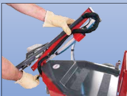
Simple and easy to fold, pull out the bolt and fold down handle.
